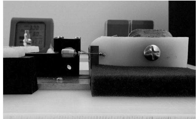
Figure 1. The flexural fatigue testing model
