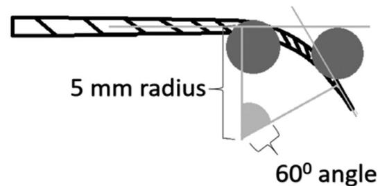
Figure 2. Each instrument was constrained to rotate at a 60° angle and 5 mm radius of curvature
