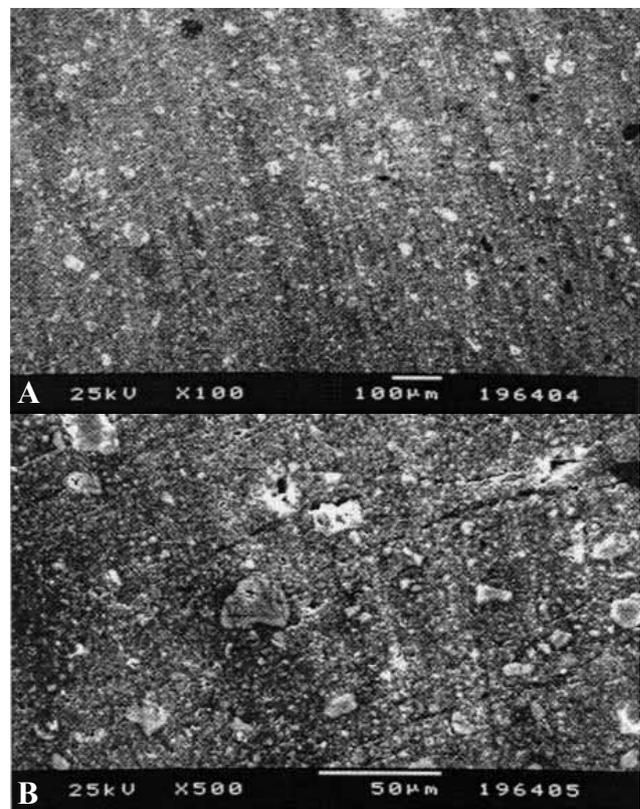
Figure 3. Scanning electron micrographs depicting surface profiles of Surefill (magnification: A - x100; B - x500)
