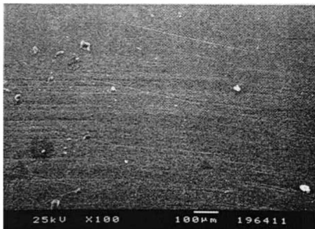
Figure 4. Scanning electron micrograph depicting surface profiles of Z100 (magnification x100)
