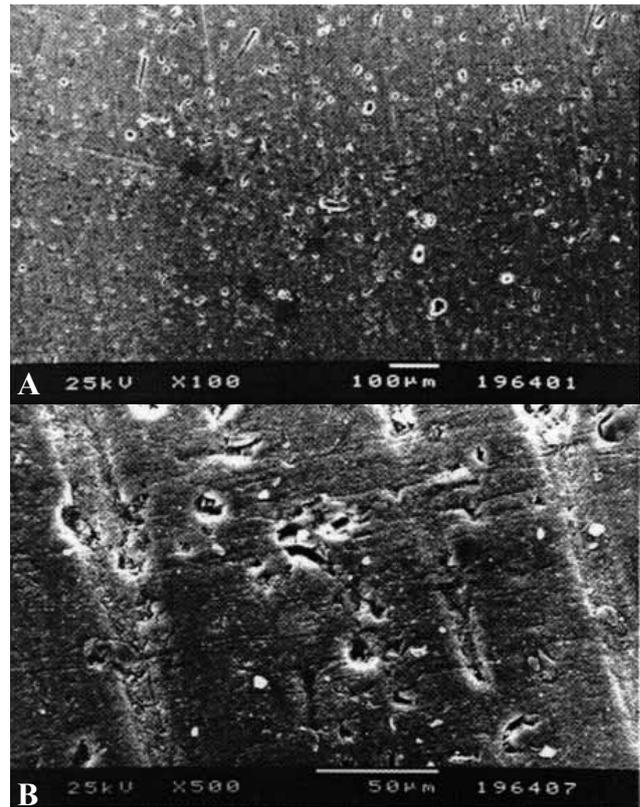
Figure 2. Scanning electron micrographs depicting surface profiles of Alert (magnification: A - x100; B - x500)
