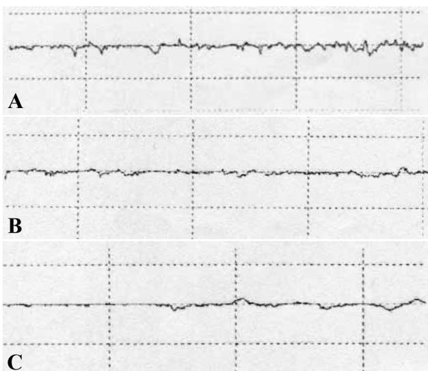
Figure 1. Surface profile tracing of composites finished and polished (A - Alert; B - Surefill; C - Z 100)
