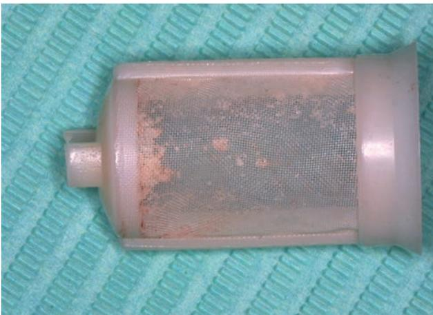
Figure 2. Collection of bone during high speed drilling from the filter
