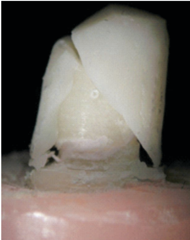
Figure 3. IPS e.max Press fractured crown over Y-TZP VALLPOST BO-S (Ø 1,6mm) with press core
