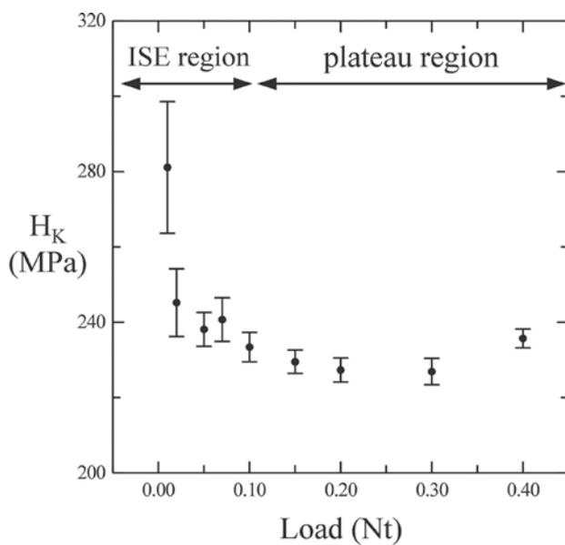
Figure 2. Schematic illustration of Vickers microhardness ( $H_v$ ) as a function of the applied load, where the ISE and the Plateau areas are depicted for the VVS beads. The error bars represent the mean standard deviations
