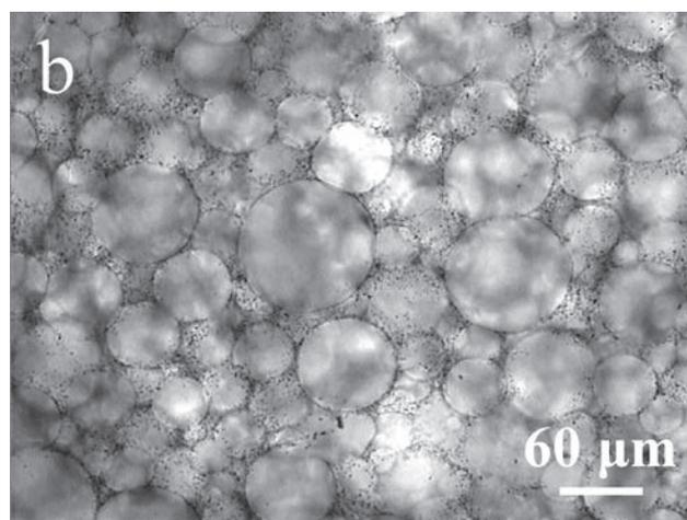
Figure 1b. Optical micrograph illustrating the morphology of the as-supplied Vita inner teeth. The PMMA beads are, here, well defined and clearly distinguishable within the cross-linked polymer matrix
